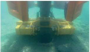
The funding from OWGP enabled Leask Marine to successfully demonstrate the operation of its submersible drilling rig and anchoring solution, and obtain third party verification validating the loads obtained. The results highlighted the opportunites for low-cost rock anchoring solutions in Offshore Wind, and confirmed the company's potential in the sector.
