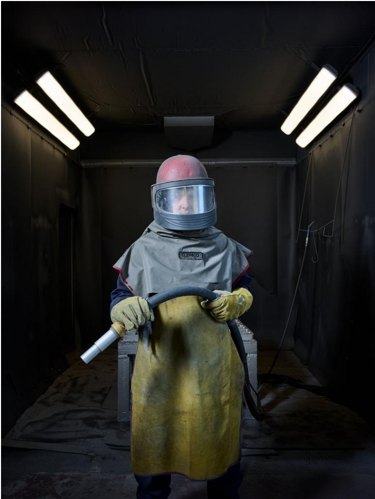
Above: image shows a grit blaster ready to clean and prepare the surface of a cast component
