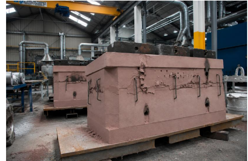
Above: airset moulding casting employs chemically bonded sand that cures at room temperature, making it suitable for larger and heavier castings.
