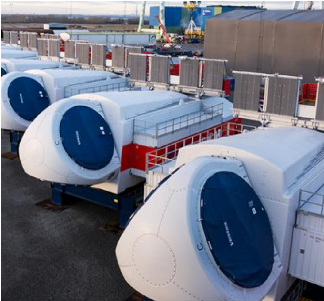
Above: Vestas nacelle and hubs after assembly. Image courtesy of Vestas
