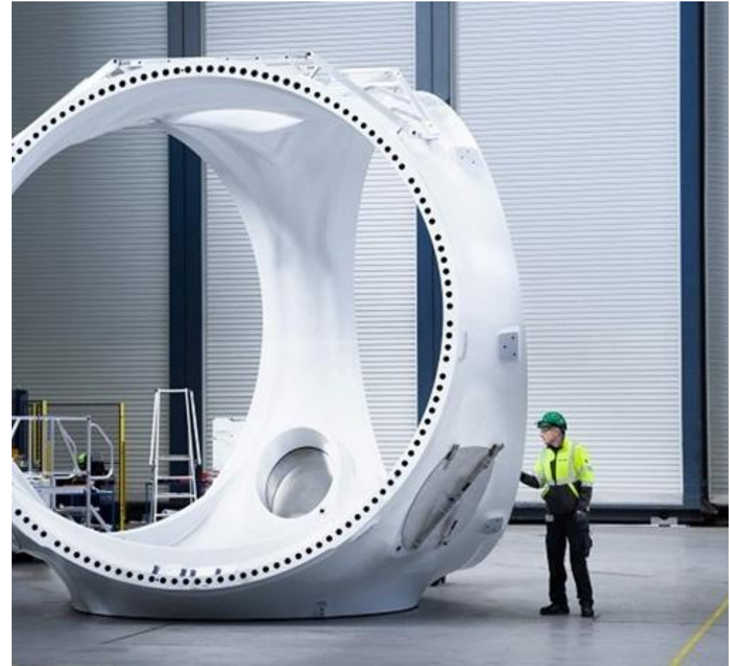
Above: a Vestas V236 cast hub body. An individual hub casting will be approx. 50 tonnes, meaning only a few specialist foundries in Europe can supply. Image courtesy of Vestas
