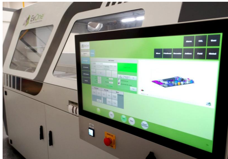
Left: 3D sand printing for sand moulds and cores for prototype and production metal castings. 3D printing allows rapid prototyping without costly tooling and cost-effective production of smaller castings.
