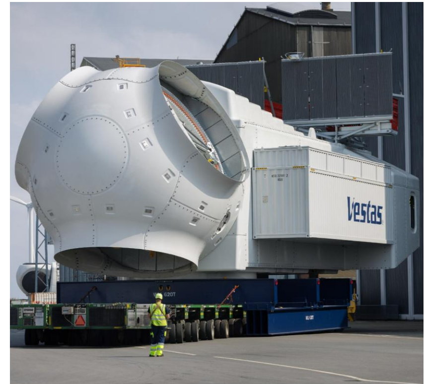
Above: a Vestas V236 nacelle and hub is moved on an SPMT. Image courtesy of Vestas
